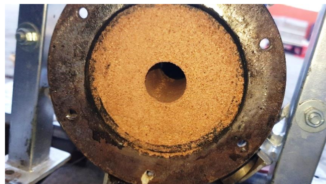
Figure 7. Date stone biomass fuel grain installed in a combustion chamber.
