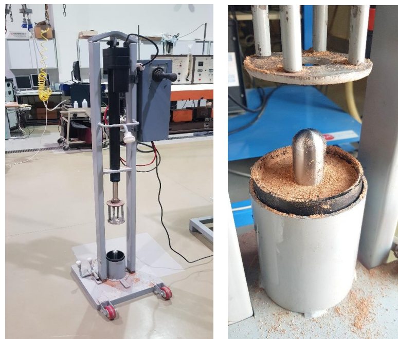
Figure 6. Compression device whole structure (left) and biomass fuel compressed (right).
