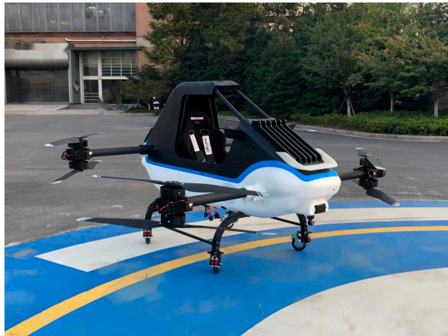
Figure 1. Image of eVTOL aircraft with a maximum takeoff weight of 350 kg. The maximum forward speed is 60 km/h and the endurance is 35 min. The payload is 80 kg and seats 1 person.
