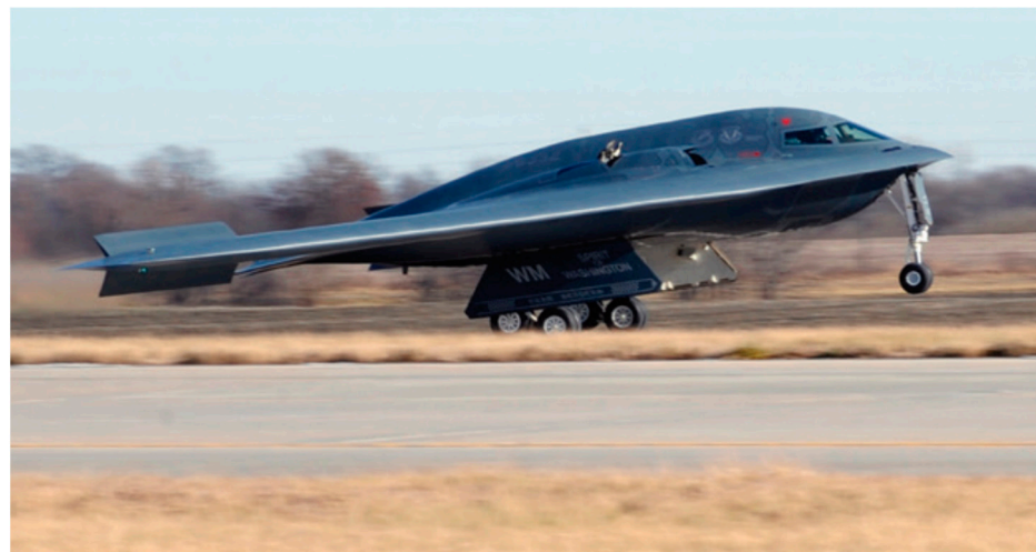
Figure 11. Split drag rudders on B-2 Spirit. Courtesy of the U.S. Air Force.
