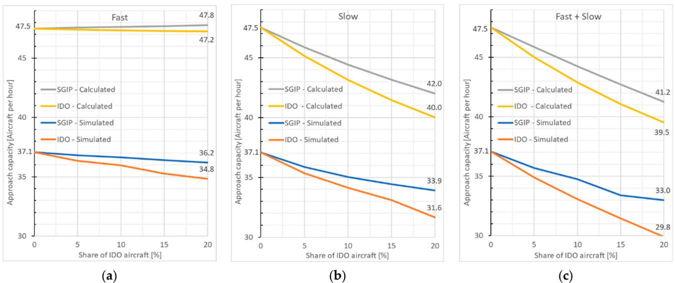
**Figure 13.** Approach capacity with increasing shares of (a) Fast (20 kts faster), (b) Slow (40 kts slower), and (c) Fast + Slow traffic. The two upper graphs show the difference between IDO and SGIP scenarios in a calculated optimized environment. The lower two graphs show the difference between IDO and SGIP for a specific scenario, simulated with BlueSky.
