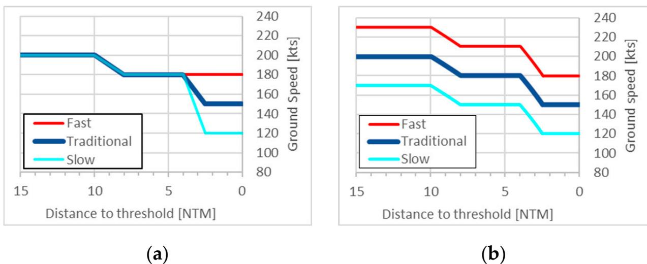
**Figure 6.** Fast, Traditional, and Slow speed profiles used for the calculations with 30 kts speed difference (as an example of a speed difference). Within the baseline, all aircraft maintain the same restrictive speed schedule until they have to reduce (or maintain) their speed for final approach speed (a). Within all future scenarios (IDO and SGIP) the approach speed is selectable and maintains a constant off-set based on the selected profile throughout the entire last 15 NTM (b).
