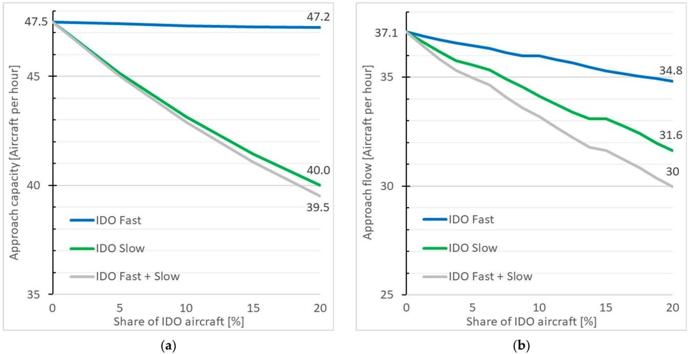
**Figure 12.** Calculated (a) and with BlueSky simulated (b) capacity for increasing shares of IDO traffic for Fast aircraft (20 kts speed difference), Slow aircraft (40 kts speed difference), and Fast + Slow. The difference of approximately 10 aircraft per hour between (a,b) is caused by traffic pressure gaps within the baseline of the simulation.
