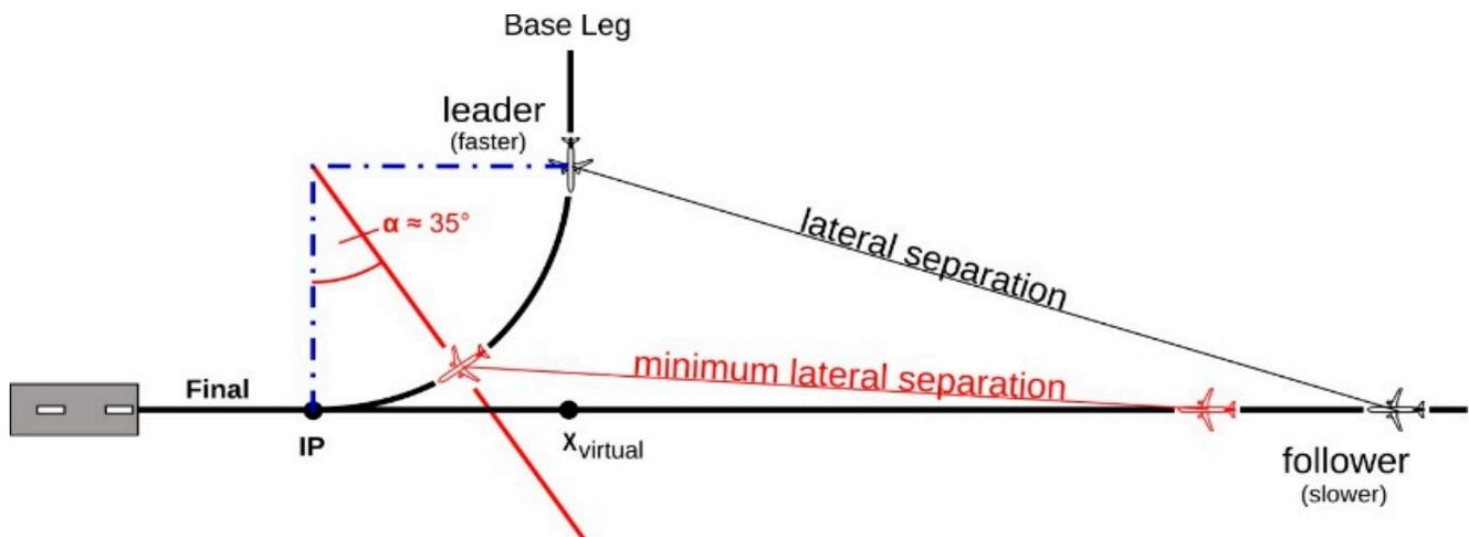
Figure 7. Moment of minimum lateral separation for Case 2 and the Fast—Slow aircraft pair.
