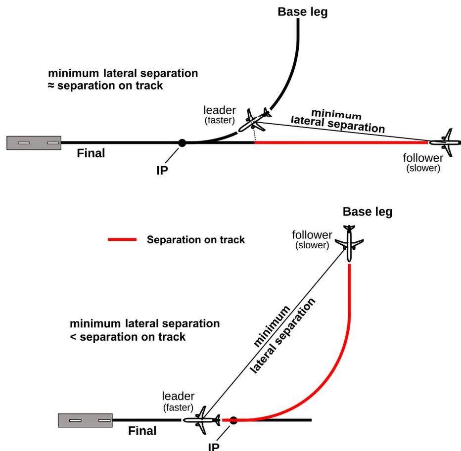
**Figure 8.** Graphic illustration of the geometric advantage of guiding faster aircraft via the IP on final (top of the two figures). Clearly recognizable is the shorter separation on track to obtain the same separation laterally. In the case of the slower aircraft via IP, there is a significantly different geometric constellation at the time of minimum separation.
