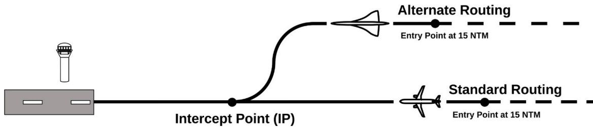
**Figure 2.** Concept drawing of the SGIP. The alternate Routing offers a deemed separated approach path to the standard routing via lateral separation. The concept study starts at an entry point at 15 NTM.
