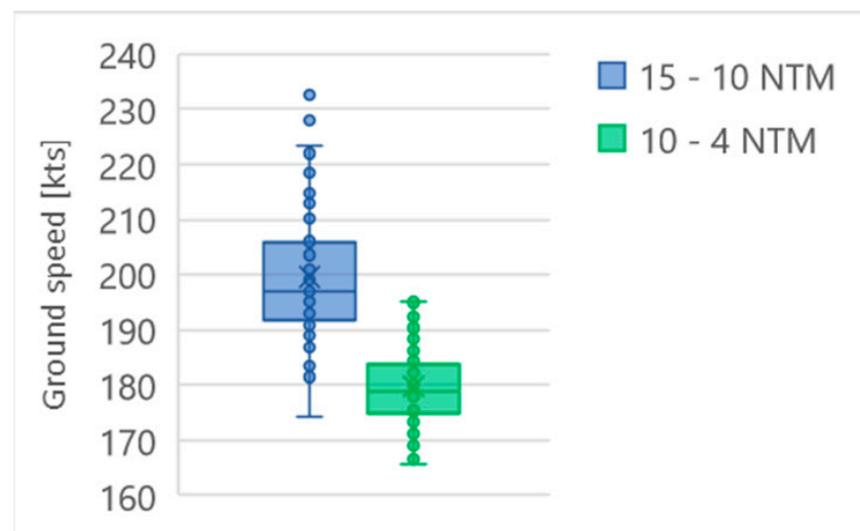
**Figure 5.** Speed data from the ADS-B dataset within the baseline scenario and the resulting average speeds of aircraft between 15–10 NTM and 10–4 NTM.
