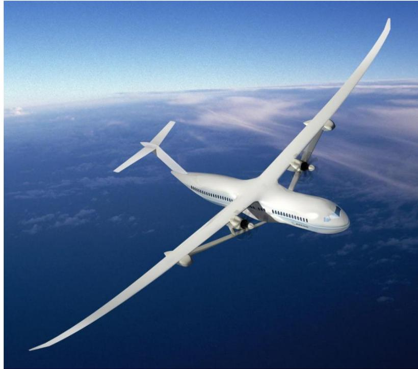
**Figure 2.** Configuration of a Boeing Transonic, Truss-Braced Wing (image credit: NASA/The Boeing Company [14]).
