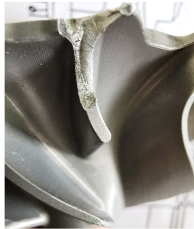
Figure 14. Photograph of the damaged turbine impeller.
