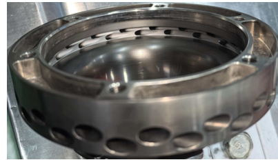
Figure 4. Photograph of tubular nozzles with the double-row staggered layout.
