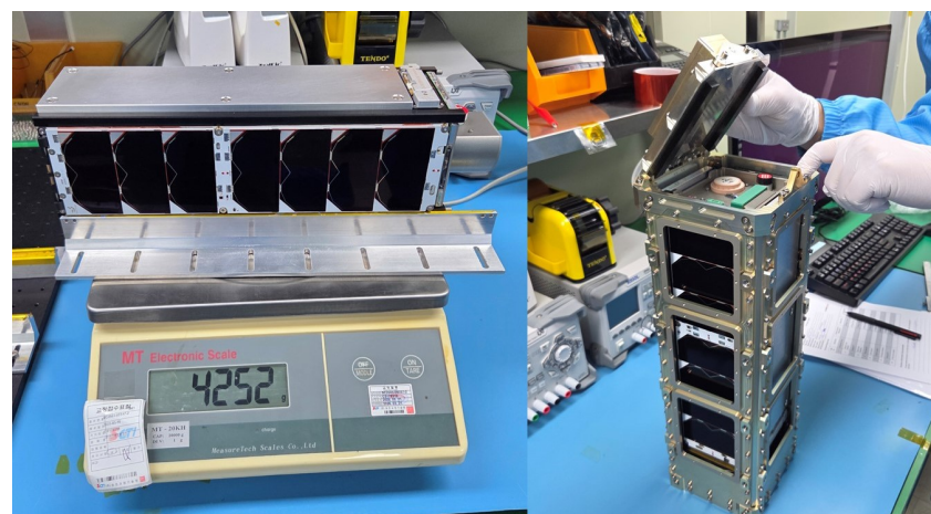
Figure 7. Mass measurement and deployer interface verification of the fully assembled COSMIC flight model before launch accommodation.
