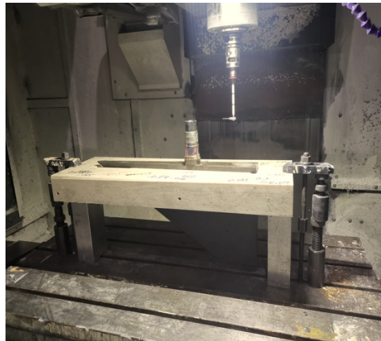
Figure 9. Physical installation diagram of trigger probe on CNC machine tool.
