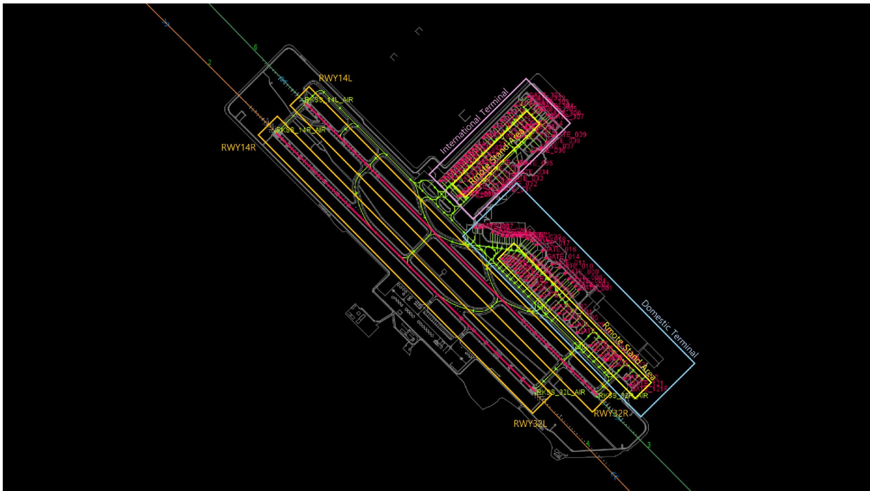
Figure 3. Simulation model of the ground operations at Gimpo International Airport.
