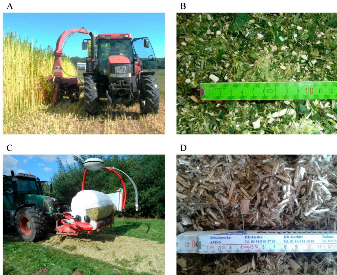
Figure 2. Harvesting of hemp with forage harvesters (A) for subsequent wet preservation storage (C), fresh chopped hemp whole crop material (B), wet preserved hemp whole crop material (D).
