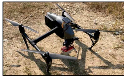
Inspire DJI (attached with Micasense multispectral)
