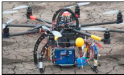
Mikrokopter JR11X (attached with multispectral MCA 6)
