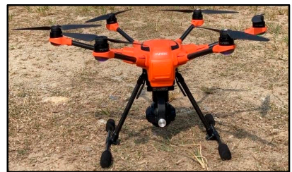
Yuneec H520 hexacopter (attached with thermal sensor)
