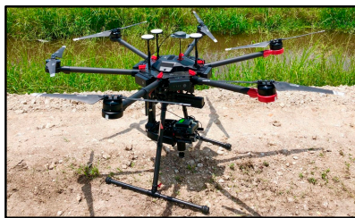
Matrice 600—DJI (attached with Hyperspectral Pika L)
