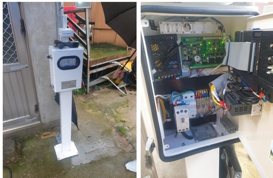
**Figure 2.** The outside and inside of livestock odor management system. The sensor case (outside) must protect the inside, and the inside is composed of a measurement sensor, modules, communication equipment, and power terminal.
