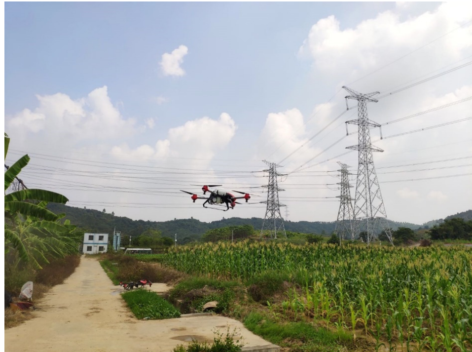
Figure 17. Agricultural drone sprays herbicides on corn fields. Copyright source: own work.
