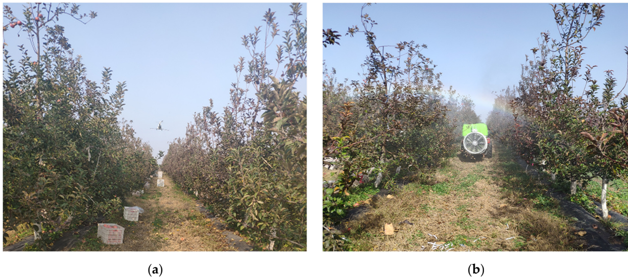
Figure 15. Agricultural spraying machinery working in the orchard. (a) Single-rotor oil-powered UAV; (b) round orchard wind-driven sprayer [82]. Copyright source: reproduced from [A comparative study on the performance of single-rotor oil-propelled UAV and circular air-fed orchard sprayer], with permission from Yongliang Bian, 2021.
