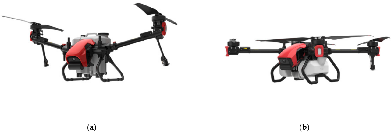
Figure 21. XAG's new agricultural UAV of 2021. (a) V40 with double-rotor [104]; (b) P80 with a load capacity of 40 kg [105]. Copyright source: reproduced from ( https://www.xa.com/v40-2021 (accessed on 20 January 2022), https://www.xa.com/p80-2021 (accessed on 20 January 2022)), with permission from XAG, 2021.
