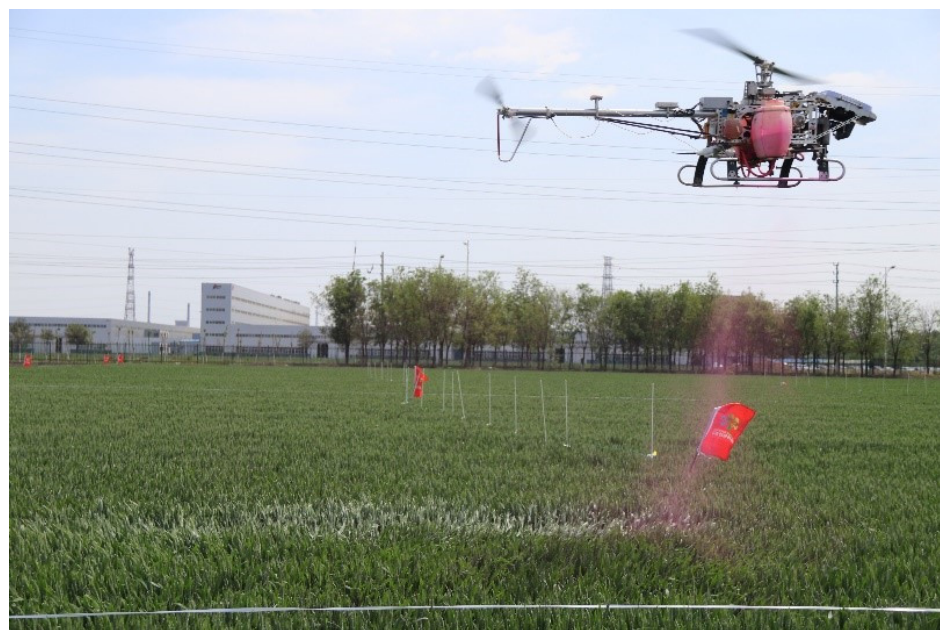
Figure 8. Agricultural UAV sprays pesticides on rice. Copyright source: own work.
