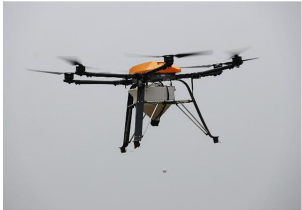
Figure 18. Agricultural drone drops the Trichogramma capsule. Copyright source: own work.
