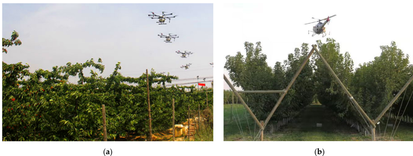
Figure 16. Operating status of different UAVs over cherry trees. (a) Agricultural UAVs perform autonomous flight and coordinated spraying on cherries [88]; (b) Test cherry trees are trained to Y-trellised canopy architecture. During field trials, the unmanned middle-size helicopter flies above the canopy at different altitudes and speeds [89]. Copyright source: (a) reproduced from ( http://www.chengcheng.gov.cn/ccdt/dzdt/38397.htm (accessed on 20 May 2019)), with permission from Chengcheng Country People's Government, 2019. (b) reproduced from [Efficacy of unmanned mid-sized helicopter in rainwater removal from cherry canopies], with permission from Elsevier, 2021.
