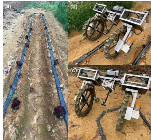
Figure 10. The appearance of experimental field and the two-wheeled robot: (a) the appearance of the field; (b) the snapshot of the two-wheeled trailer traveling autonomously; (c) the U-turning process of the robot trailer.
