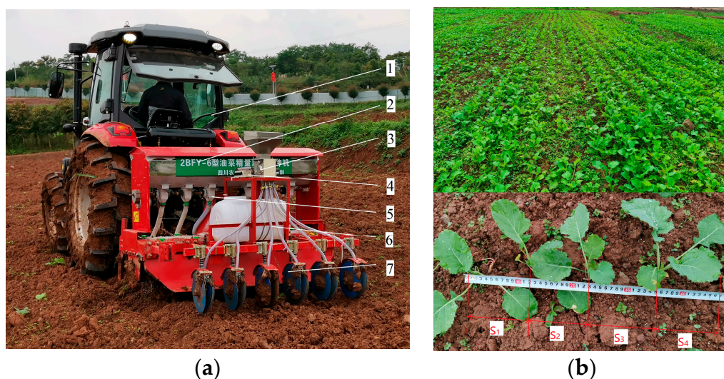
Figure 6. Field experiment of the rapeseed seeder (a) and seedling growth and measurement (b). Note: (1) tractor, (2) fertilizer box, (3) centralized seed-metering device, (4) controller, (5) fertilizer-metering device, (6) seed tube, and (7) double-disc opener.
