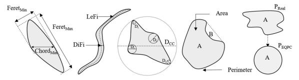
**Figure 2.** Schematic representation of particle size and shape assessment (Equations (1) to (5)) derived from the calculation of diameters (Feret<sub>MIN</sub>, Chord<sub>MIN</sub>, Feret<sub>MAX</sub>, DiFi [diameter of fiber], LeFi [length of fiber], D<sub>CC</sub>), area, and perimeter assessed by dynamic image analysis.
