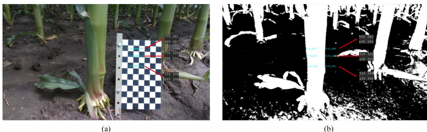
Figure 6. The process of measuring the stem diameter of maize: (a) pixel width of the square and (b) pixel width of maize stem.
