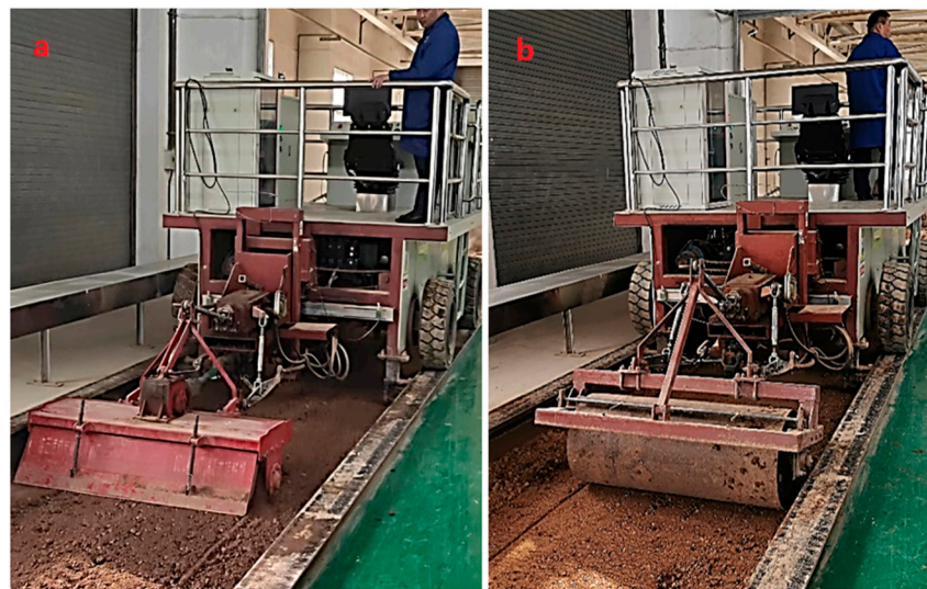
Figure 5. Preparing the soil bin: (a). Mixing the soil with a rotary tiller; (b). Compacting the soil with a cylindrical roller.
