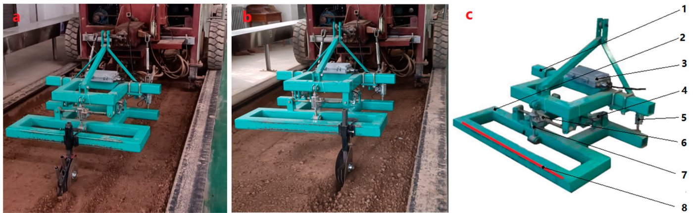
Figure 6. Measuring horizontal and vertical forces with a volumetric dynamometer unit: (a). Testing designed double disc colter; (b). Testing base double disc colter; (c). Volumetric dynamometer unit parts; 1. Upper frame; 2. Bottom frame; 3. CAN bus system; 4. Horizontal right load sensor; 5. Vertical right load sensor; 6. Lateral load sensor; 7. Back vertical load sensor; 8. A place to mount colters.
