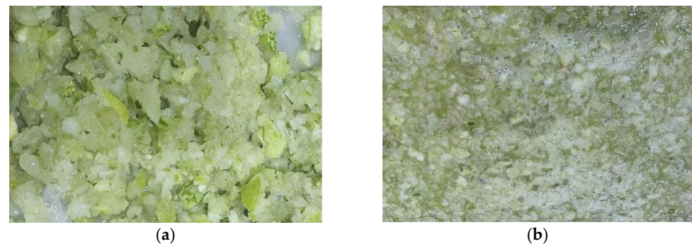
Figure 16. The crushing effect of the seed-used watermelon rind. (a) The crushing effect under the original parameters; (b) the crushing effect after parameter optimization.
