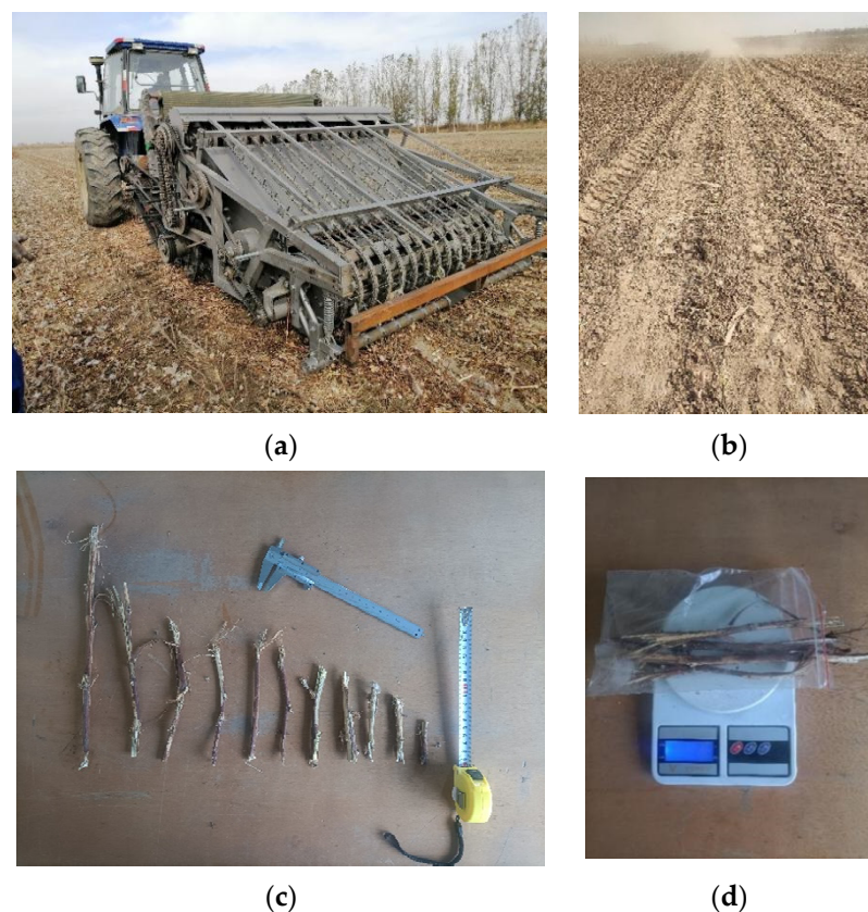
Figure 19. Field trial. (a) Proof test. (b) Surface after operation. (c) Screening of unqualified cotton stalk crushing. (d) Measurement of qualified rate of cotton stalk crushing.
