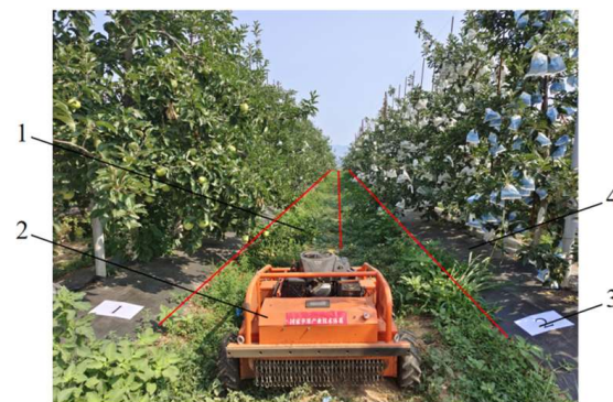
Figure 9. Orchard testing site: 1. Job line. 2. G301. 3. Job line number. 4. Ground cloth. The red line represents the dividing line of the homework line.
