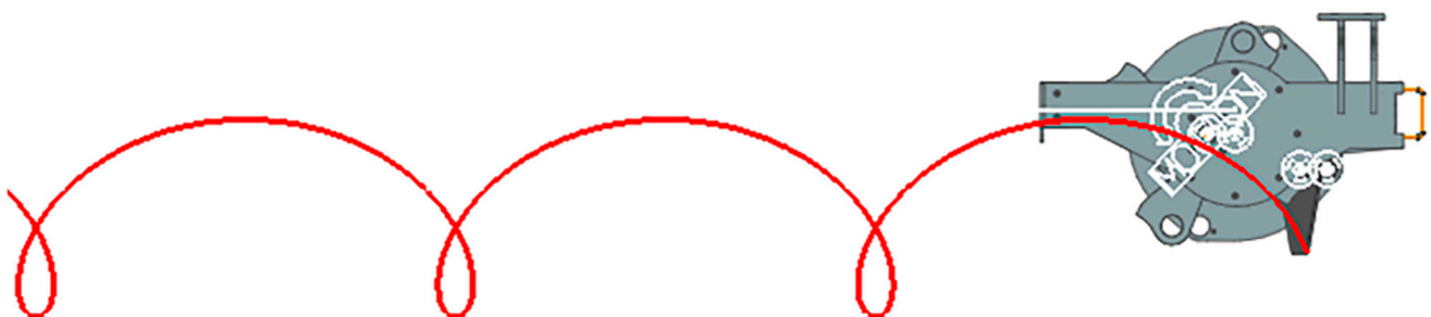
Figure 15. Simulation of the trajectory of the drilling and seeding tip for a 20-tooth sprocket.
