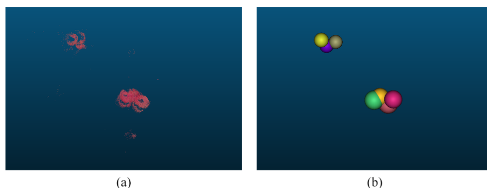
Figure 10. Results of the tomato fruit point cloud extraction and spherical fitting: (a) shows the extracted point cloud of the tomato fruits, and (b) shows the result after spherical fitting of the tomato fruit point cloud.
