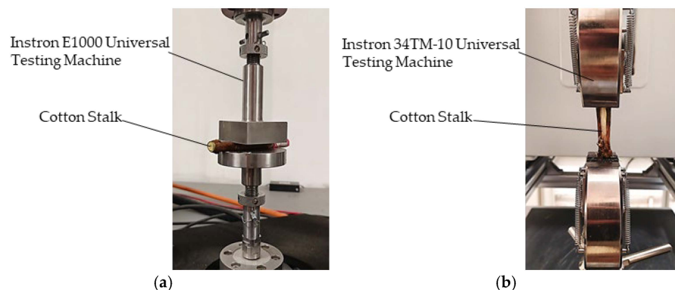
Figure 1. Cotton stalk force analysis diagram. (a) Cotton stalk compression process. (b) Cotton stalk stretching process.
