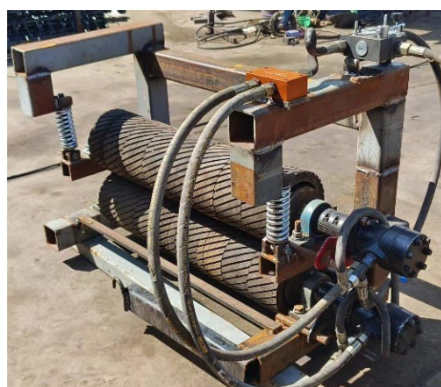
Figure 8. Clamping Mechanism for Horizontal Shaft Counter-Rolling Cotton Stalk Extraction Machine.
