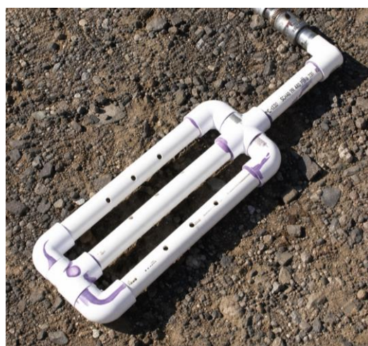
Figure 8. Air-flow cushioning collection device for reducing fruit falling velocity and maintaining fruit spacing during mechanical vibration harvesting [25].
