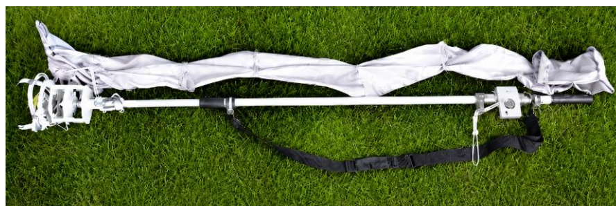
Figure 6. Manually operated backpack-type pear picker used to reduce repeated climbing and manual fruit transfer during pear harvesting [21].
