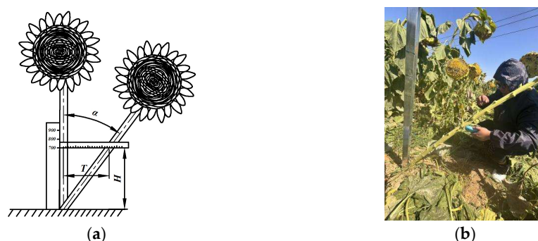
Figure 2. Schematic diagram of the critical bending angle measurement for edible sunflower. (a) Diagram of measurement. (b) Site survey blueprint.
