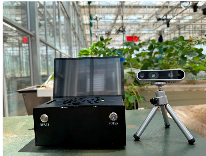
Figure 11. Edge deployment device and RGB-D sensor used in the experiment.
