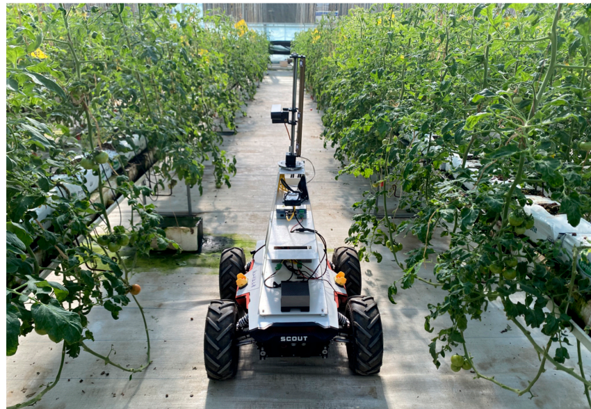
Figure 2. The SCOUT 2.0 autonomous mobile platform operating in the greenhouse environment. The platform traverses the ridges to simulate the trajectory of robotic harvesting under real-world unstructured conditions.
