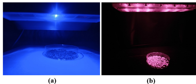
Figure 1. Laser irradiation setup: (a) blue light irradiation; (b) red light irradiation.
