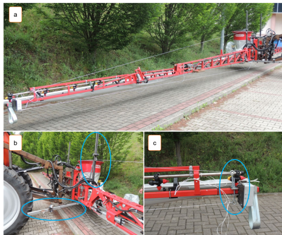
Figure 4. Measurement system for evaluating sprayer boom displacement from the equilibrium position. (a) General view of the boom displacement measurement system; (b) support arms equipped with reel spools and cable tension springs; (c) loop screws used for attaching the measuring cables. Adapted from Ref. [42].
