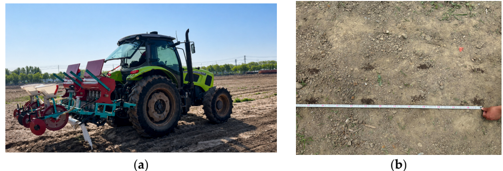
Figure 12. Field Experiment: (a) Performance test of the planter; (b) Hole fertilization operation effect.
