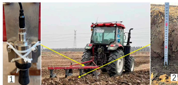
Figure 12. Field test scenario. 1. Ultrasonic sensor, and 2. manually measured tillage depth.
