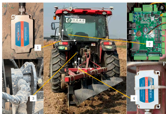
Figure 1. Test platform for tillage depth monitoring system. 1. Tractor-mounted IMU; 2. industrial control board; 3. angle sensor; 4. And plough-mounted IMU.
