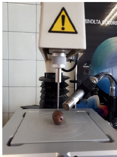
Figure 2. Needle test by TA.XT Plus Texture Analyzer.
