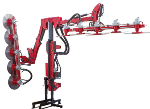
Figure 2. V-DUAL ID-PLUS multifunctional pruning machine (source: Industrias David S.L.U. [22], adapted).
