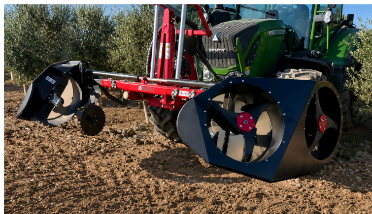
Figure 1. OLIX-S under-canopy skirting pruner mounted on the tractor during field operation in an intensive olive orchard (source: Industrias David S.L.U. [21], adapted).
