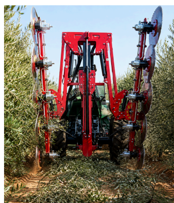
Figure 3. V-DUAL ID-PLUS multifunctional pruning machine during operation.
