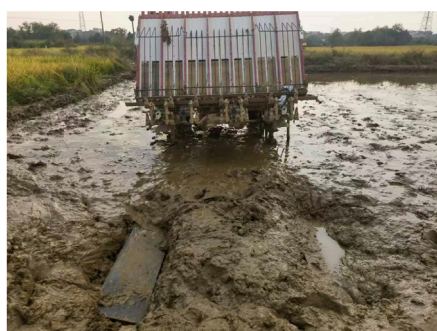
Figure 14. On-site layout of the sideslipping device.
