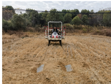
Figure 10. On-site experiment for slip identification on dry farmland.
