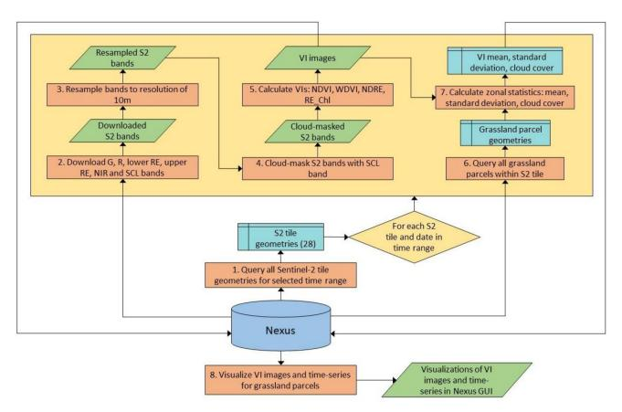
**Figure 2.** Flowchart containing processes for querying, harvesting, pre-processing, uploading, and visualizing Sentinel-2 (S2) data and vegetation indices (VI) for each S2 tile of  $100 \times 100 \text{ km}^2$  and date in time range, as part of the Sen2Grass system, with the Nexus server as a central geodatabase.
