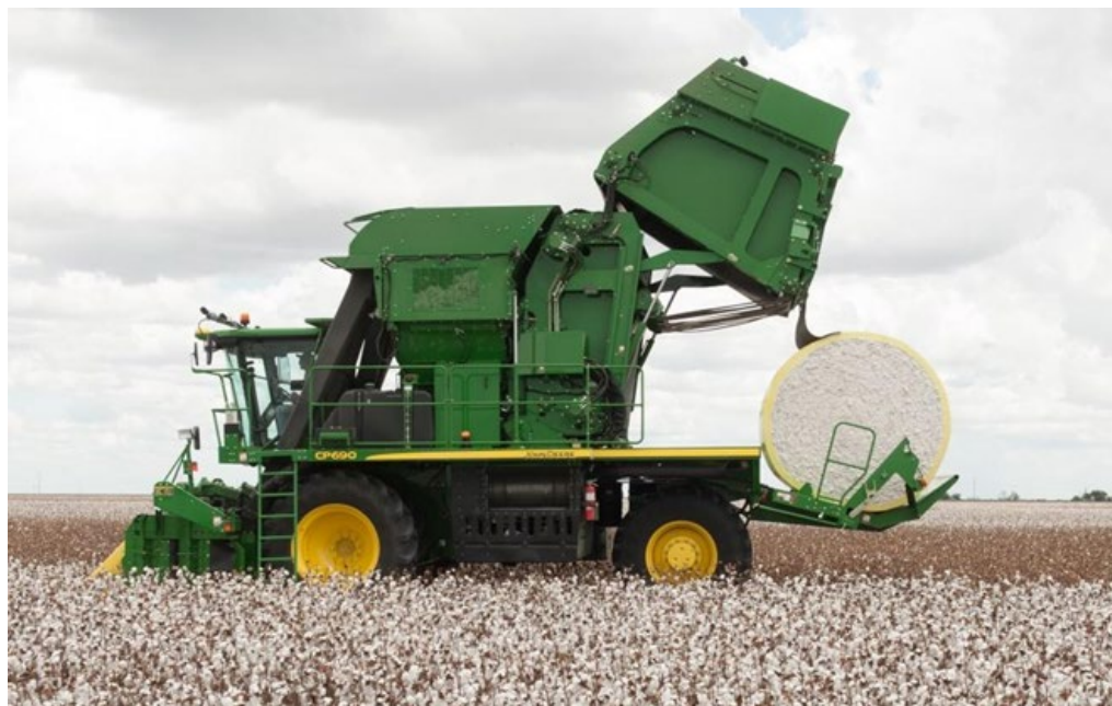
Figure A2. A module building spindle cotton harvester (often referred to as a “picker”).
