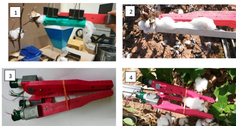
Figure 2. Image 1: one-finger end-effector; image 2: one-finger end-effector; images 3 and 4: three-finger end-effector [73]. Adapted from Gharakhani and Thomasson (2021).
