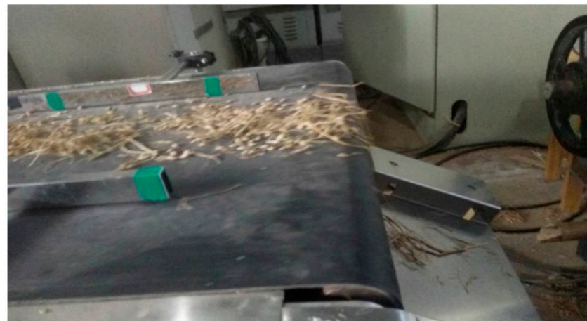
Figure 21. Experimental test bench of grain/MOG falling on the sensor plate [7].
