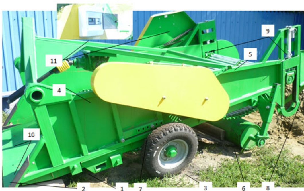
Figure 16. General view of a machine for harvesting root crops and onions, equipped with a separating rod elevator with an adjustable angle of inclination of the web: 1, frame; 2, digging ploughshare; 3, support wheels; 4, main separating rod elevator; 5, additional rod elevator; 6, roller-bed-forming machine; 7, adjusting plate of the shaker; 8, narrowing tray; 9, electric cylinders; 10, weight sensor of the digging ploughshare; 11, microcontroller.
