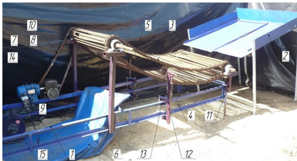
Figure 11. A general view of a laboratory installation for determining the effect of the technological parameters of a separating rod elevator on the quality indicators of the separation of a pile of root crops (bulbs): 1 frame; 2 container for preliminary placement of the pile; 3 separating rod elevator; 4 elliptical shaker; 5 supporting roller; 6 tarpaulin of separated products; 7 electric motor; 8 single stage gearbox; 9 frequency converter; 10 chain transmission; 11 support racks; 12 shaker racks; 13 connecting bracket; 14 support plate; 15 network filter.
