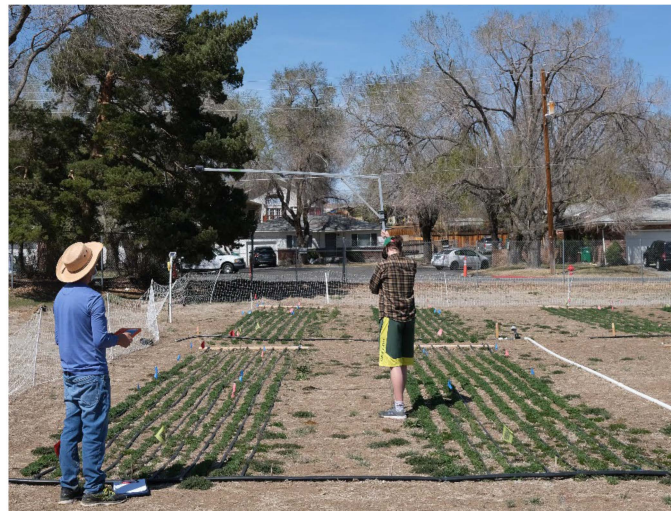
Figure 2. Multispectral camera attached to frame to acquire images. Pictures were collected inside the south, middle, and north portions of each plot, for a total of three pictures per plot.
