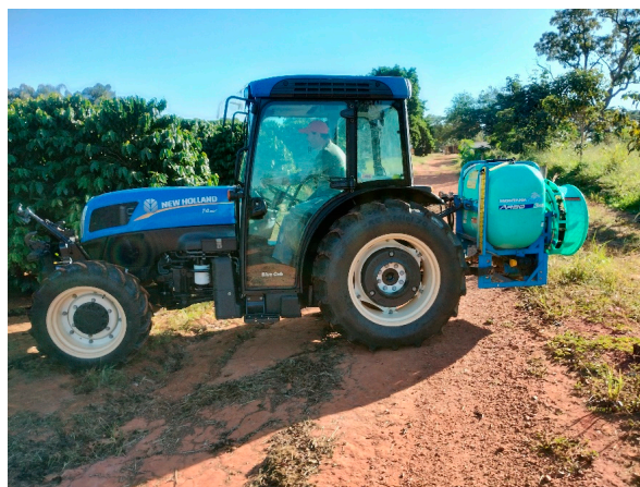
Figure 3. Airblast sprayer and tractor used for ground-based application.
