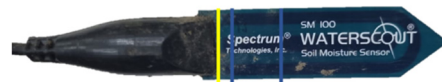
Figure 3. The photo shows a low-cost capacitive probe designed for soil moisture measurement. The yellow line indicates the “warning line”, which marks the part of the sensor that should not be inserted into the soil, while the area between the blue lines identifies the recommended depths for proper insertion into the soil.
