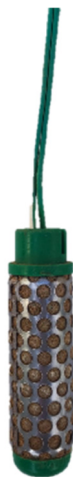
Figure 2. Granular matrix sensor, composed of a pair of electrodes embedded in a gypsum block.
