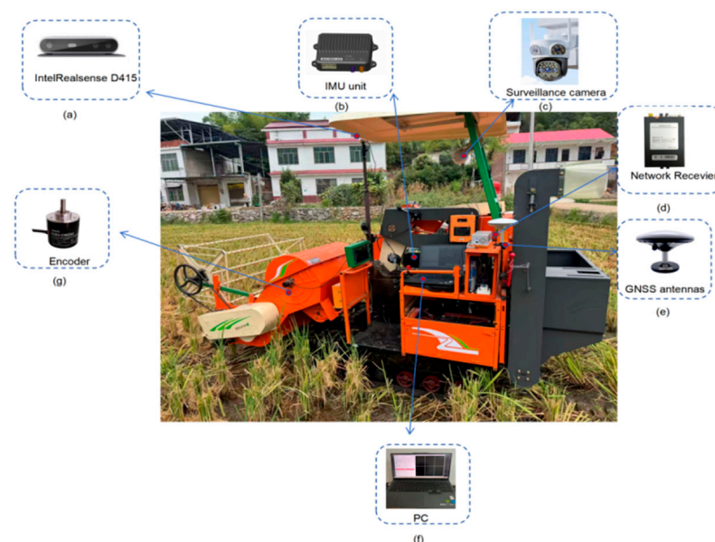
Figure 2. Whole equipment: (a) IntelRealSense D415, (b) IMU unit, (c) Surveillance camera, (d) Network Receiver, (e) GNSS antennas, (f) PC, (g) Encoder.
