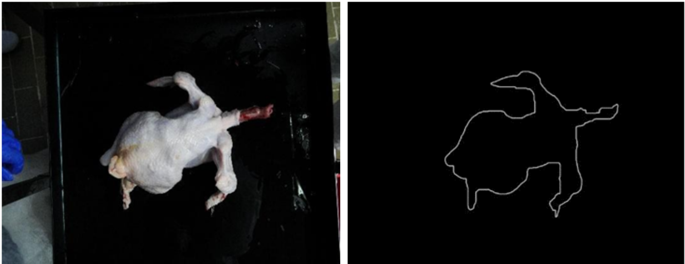
Figure 6. Example of edge-based segmentation showing fragmented contours and boundary inconsistencies under industrial acquisition conditions.
