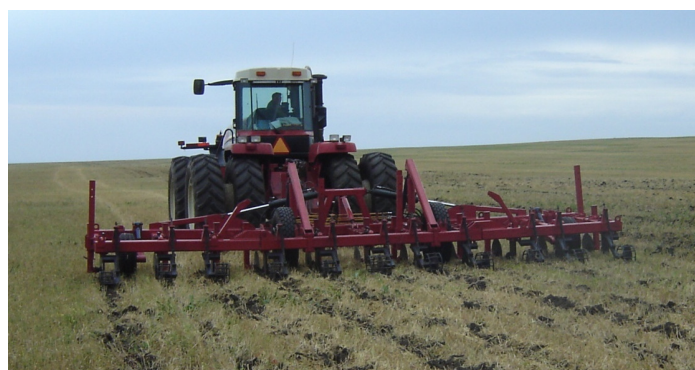
Figure 17. The unit, consisting of a “Buhler 2375” tractor and an experimental chisel implement for working on compacted and stony fields. View in operation.
