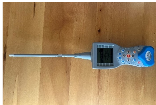
Figure 2. Instrument for measuring microclimatic factors (METREL POLY MI 6201) with the corresponding microclimatic probe.
