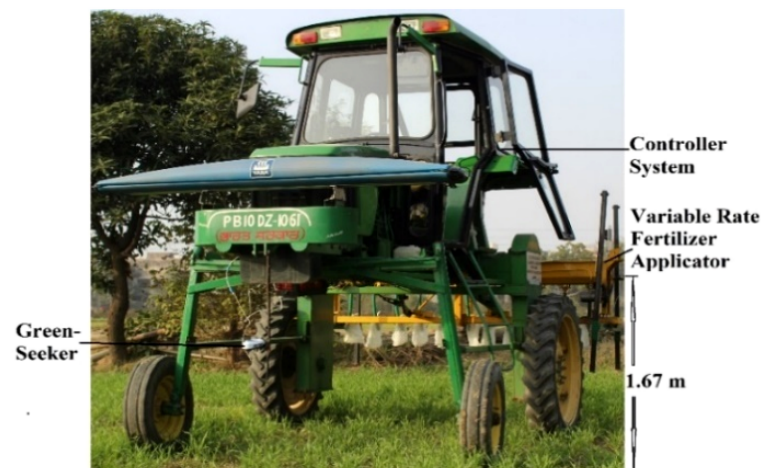
Figure 1. Archival photograph of the tractor-mounted low-cost NDVI-guided stepwise variable-rate applicator configuration, showing the active optical canopy sensor, controller, and fertilizer-metering unit. Adapted from Mirzakhani et al. [22], licensed under CC BY 4.0.
