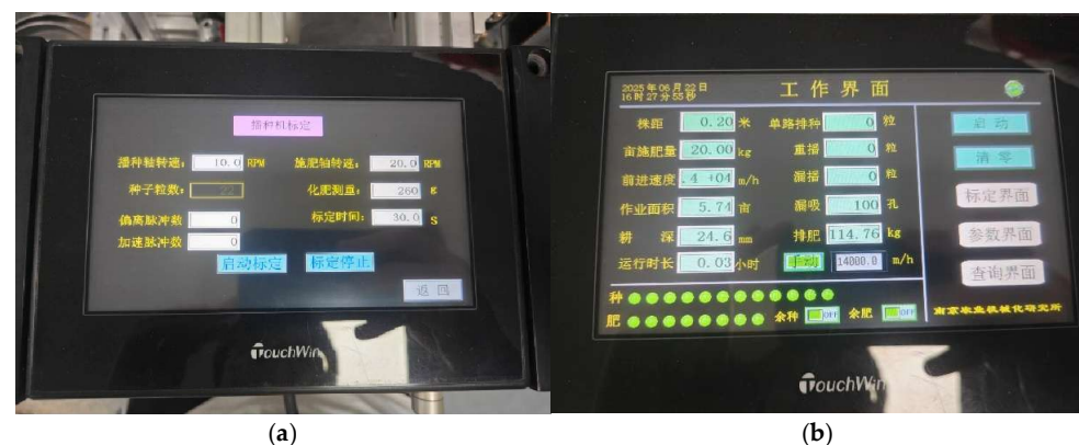
Figure 4. PLC–HMI control interfaces: (a) parameter-setting interface; (b) operating-status monitoring interface. The Chinese text shown in the photographs represents the original labels embedded in the HMI interface.
