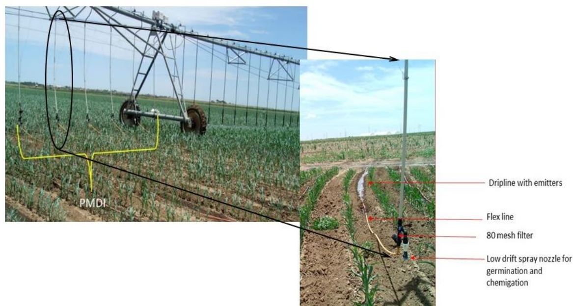
Figure 4. Precision mobile drip irrigation (MDI) system: (a) shown on span 1 to the left; and (b) zoomed-in view of one MDI drop showing sprinkler hardware, filter and dripline dragging between.
