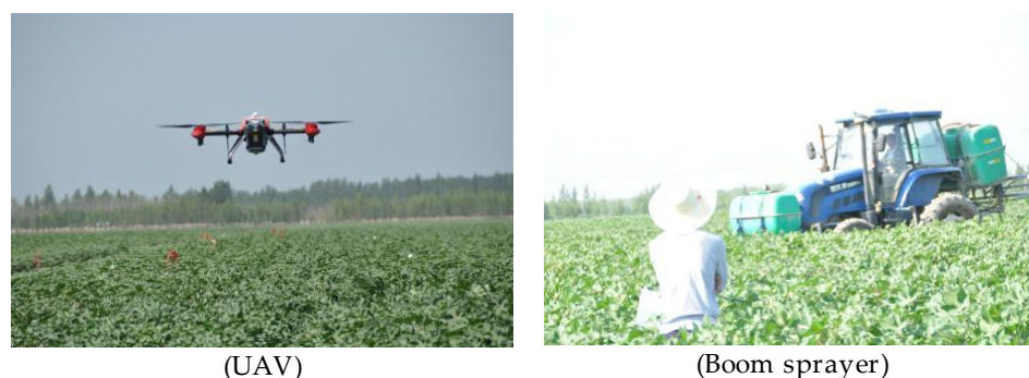
Figure 1. Unmanned aerial vehicle (UAV) sprayer and boom sprayer.
